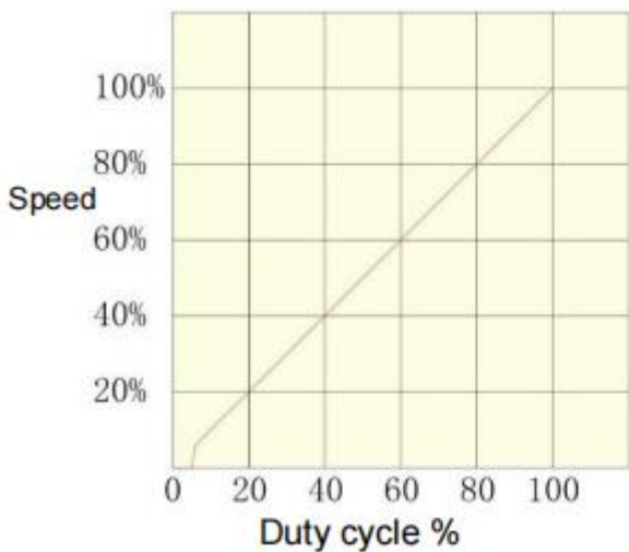
Relationship between duty cycle and motor speed (open loop no-load)
